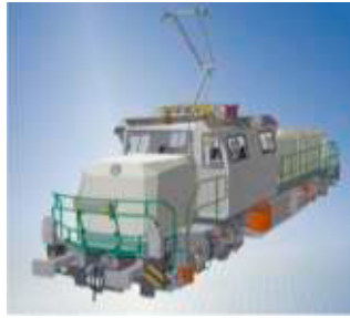
Fig. 1. Design of hybrid shunting locomotive
